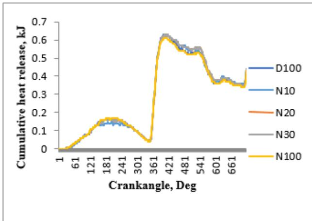
Fig. 12: Variation of cumulative heat release rate with crank angle
