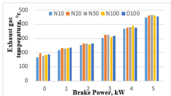
Fig. 6: Variation of exhaust gas temperature with brake power
