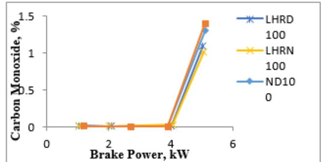
Fig. 15: Variation of carbon monoxide emission with brake power
