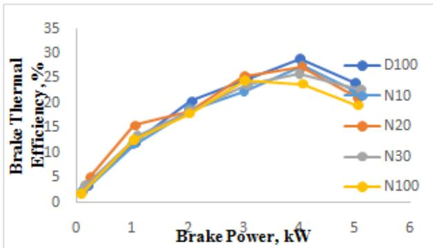
Fig. 3: Variation of the brake thermal efficiency with load for diesel and neem kernel biodiesel.
