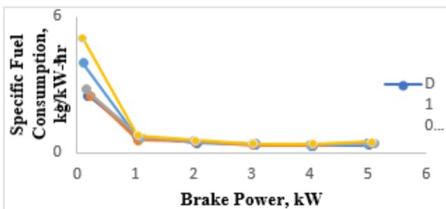
Fig. 4: Variation of specific fuel consumption with brake power.
