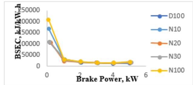
Fig. 5: Variation of break specific energy consumption with brake power
