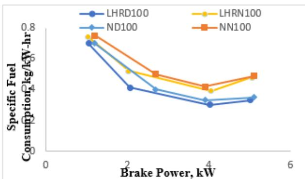
Fig. 14: Variation of specific fuel consumption with brake power
