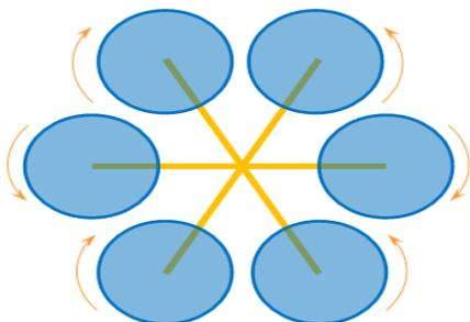
Fig. 1: General view of a “star”-airframe six-rotor helicopter
