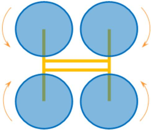
Fig. 4: General view of an H-airframe quad-rotor helicopter (model XZ-1)
