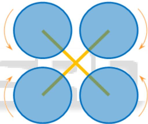
Fig. 2: Classic quad-rotor helicopter in X-configuration
