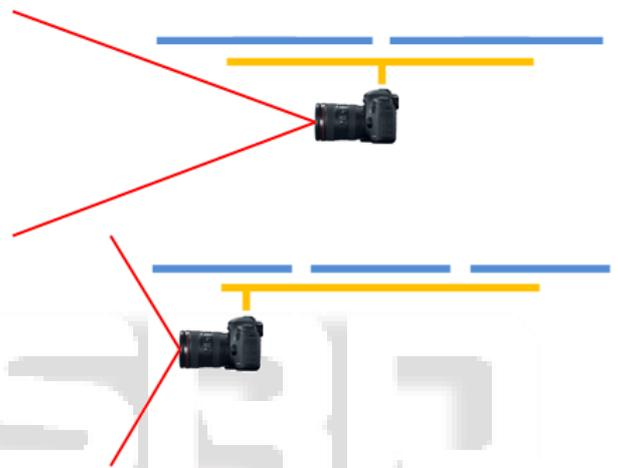
Fig. 7: Side view of “star”-airframe hex-rotor (top) and XZ-5 (bottom). The better camera position of XZ-5 is well pronounced.
