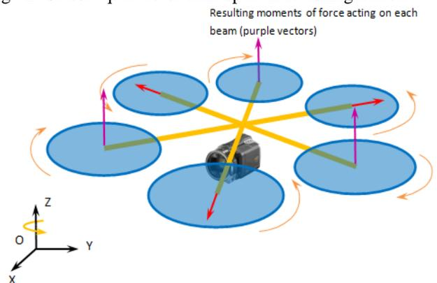
Fig. 3: Left yaw turn of a classical “star”-airframe hex-rotor helicopter
