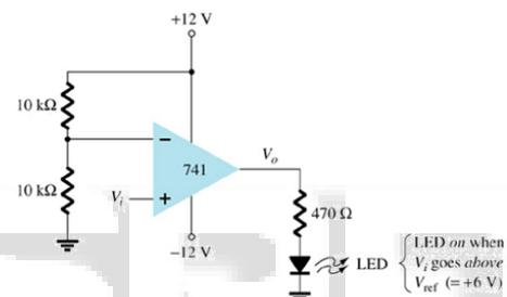
When the input  $V_i$  is greater than the reference, the output of the op-amp comparator goes high to  $+V_{SAT}$ . When  $V_i$  is less than the reference, the output is at  $-V_{SAT}$ .
