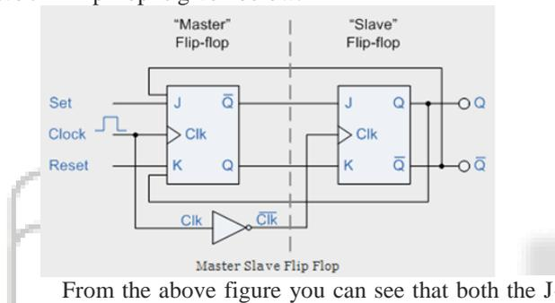
From the above figure you can see that both the J-K flip flops are presented in a series connection. The output of the master J-K flip flop is fed to the input of the slave J-K flip flop. The output of the slave J-K flip flop is given as a feedback to the input of the master J-K flip flop. The clock pulse is given to the master J-K flip flop and it is sent through a NOT Gate and thus inverted before passing it to the slave J-K flip flop.
