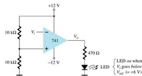
When the input  $V_i$  is greater than the reference, the output of the op-amp comparator goes low to  $-V_{SAT}$ . When  $V_i$  is less than the reference, the output is at  $+V_{SAT}$ .
