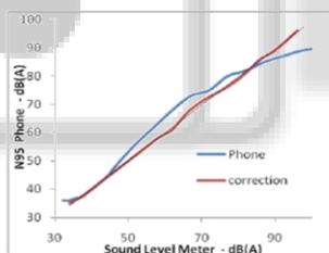
Fig. 5. Blue line: results of the distortion of the N95 phone's microphone compared to a sound level meter in the computation of the loudness ( $L_{eq}$ ). Red line: results after applying post-processing.
