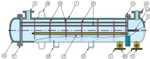
Fig. 1.1: Shell and Tube heat Exchanger construction
