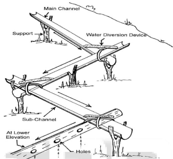
Fig. 7: bamboo drip irrigation
