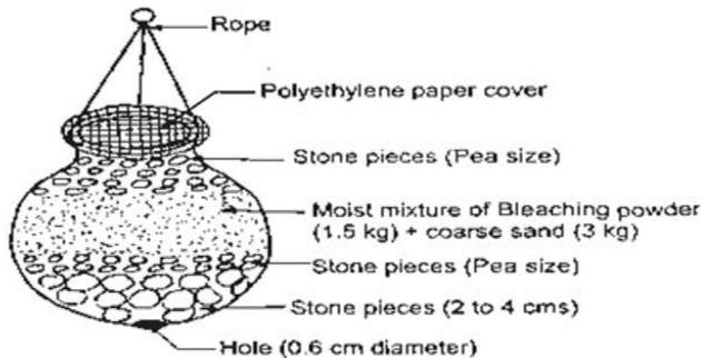
Fig. 5: The Pot Chlorinator
