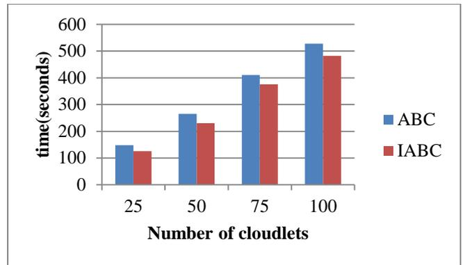
Fig. 2: Comparison of ABC and improved ABC algorithm for processing time.
