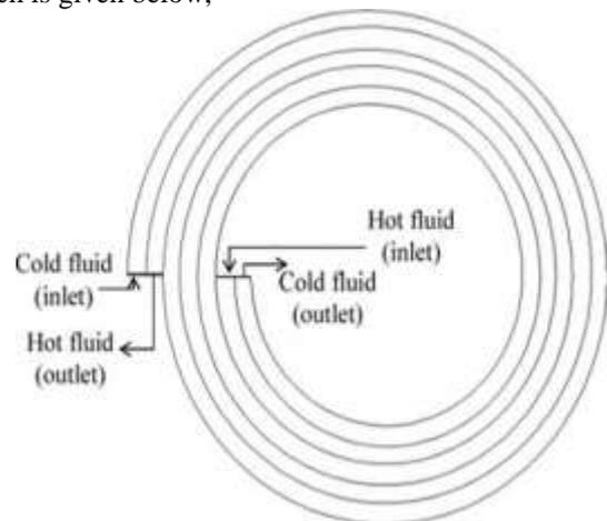
Fig. 1: Flow pattern for counter-flow arrangement in spiral heat exchangers
