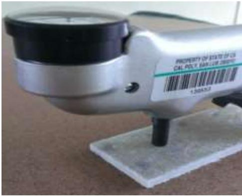
Fig. 5.1: Barcol Hardness Tester
