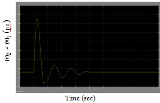
Fig. 4(a): Inter-Area Mode of Oscillation ( $\omega_2 - \omega_1$ ) for 3-Phase Fault Disturbance with SSSC
