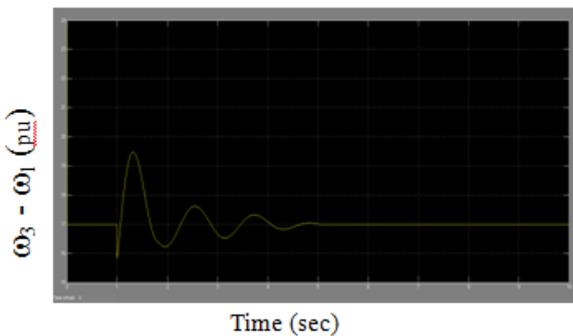
Fig. 5(a): Inter-Area Mode of Oscillation ( $\omega_3 - \omega_1$ ) for 3-Phase Fault Disturbance with SSSC
