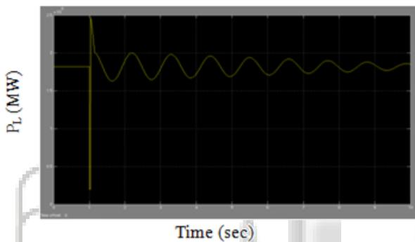
Fig. 7(b):Variation of Tie-Line Power Flow for a Three-Cycle, Three-Phase Fault Near Bus 6 Cleared by Line Tripping without SSSC
