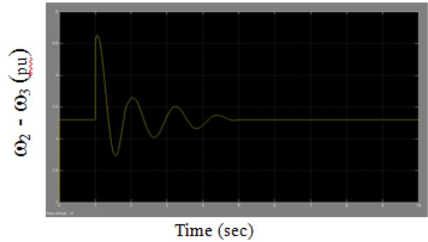
Fig. 6(a): Local Mode of Oscillation ( $\omega_2 - \omega_3$ ) for 3-Phase Fault Disturbance with SSSC
