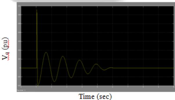
Fig. 8: SSSC Injected Voltage ( $V_q$ ) Variation for 3-Phase Fault Disturbance
