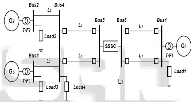
Fig. 1: Three-machine power system with SSSC
