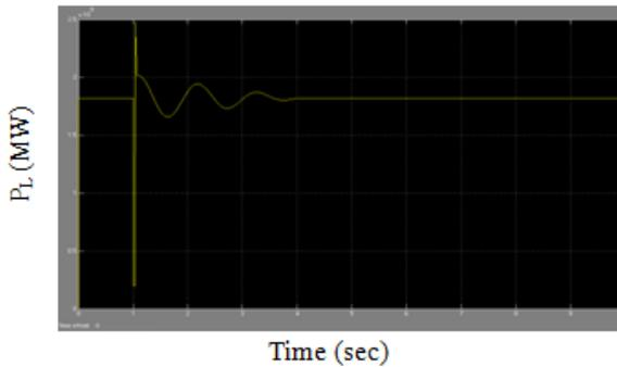
Fig. 7(a):Variation of Tie-Line Power Flow for a Three-Cycle, Three-Phase Fault Near Bus 6 Cleared by a Three-Cycle Line Tripping with SSSC
