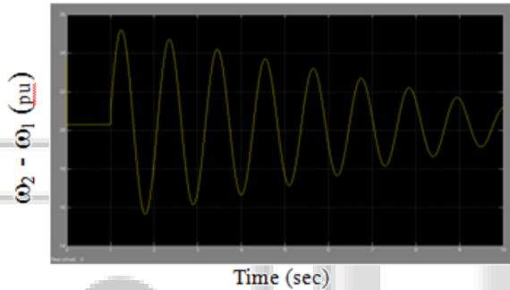
Fig. 4(b): Inter-Area Mode of Oscillation ( $\omega_2 - \omega_1$ ) for 3-Phase Fault Disturbance without SSSC
