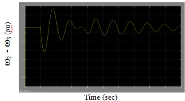
Fig. 6(b): Local Mode of Oscillation ( $\omega_2 - \omega_3$ ) for 3-Phase Fault Disturbance without SSSC
