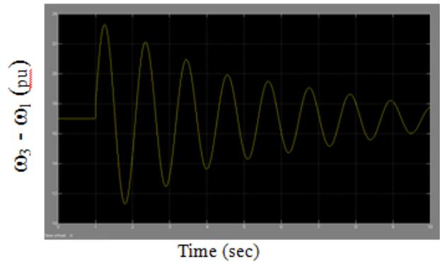
Fig. 5(b): Inter-Area Mode of Oscillation ( $\omega_3 - \omega_1$ ) for 3-Phase Fault Disturbance without SSSC
