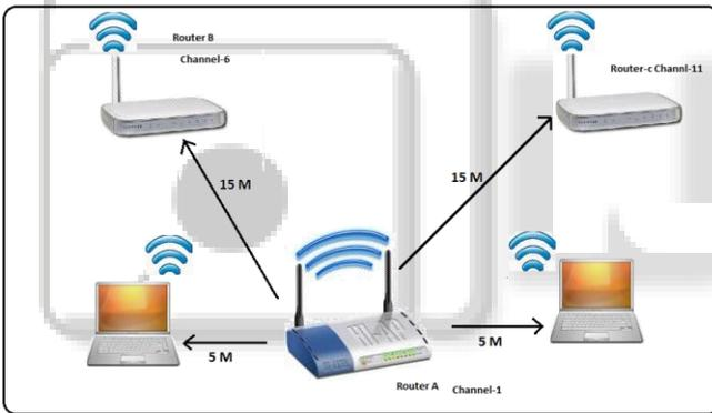
When we have increased the distance from 5 meter to 15 meter of each wireless router and increased the distance between PC1 and PC2 to 3 meter to 5 meter.
