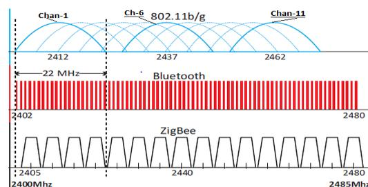
802.11, Bluetooth and ZigBee Channels in the 2.4 GHz ISM Band
