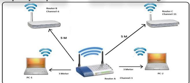
Sceniorio:- We have assign the channel-1 router A and channel-6 of router B and channel-11 router and connect the PC1 step by step each router. We observed no through put impact in the data rate transfer.
