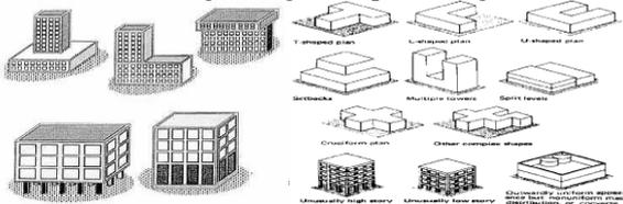
Fig. 8: Shape irregularity with causes earthquake.
