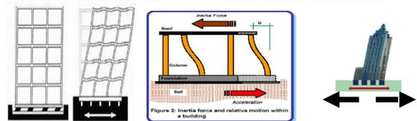
Fig. 5: Ground acceleration during Earthquake causes inertia force
