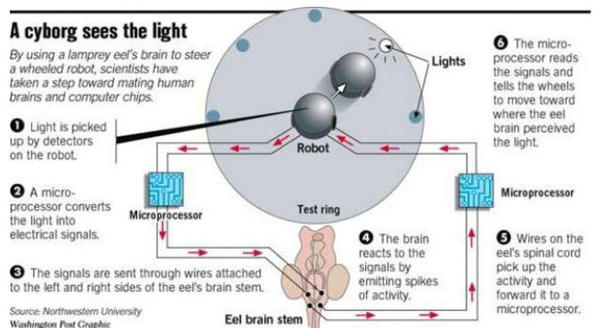
Part biological and part mechanical, the crude cyborg is equipped the brain stem of an eel, which, kept alive in a saline solution, receives input from electronic light sensors and directs the robotic wheels to move toward the source of the beam.
