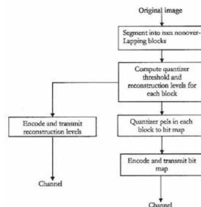
Fig. 1: Block Truncation Coding
