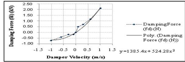
Fig. 4: Non-linear Damping Force Property of Hyundai Elantra 1992 Model Suspension Damper
