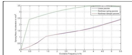
Fig.5 Sprung Mass Acceleration for Linear and Nonlinear Suspension Spring and Damper Quarter Car Model.
