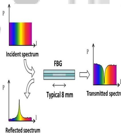
Fig. 3: Working Principle
