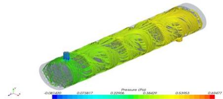
Fig. 9: Streamlines showing pressure variation for 60 kg/hr
