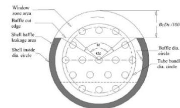
Fig. 5: Illustration of baffle cut angles, leakage area
