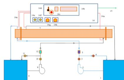
Fig. 2: Experimental set up of Shell and Tube Heat Exchanger
