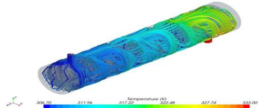
Fig. 12: Streamlines showing temperature variation for 60 kg/hr
