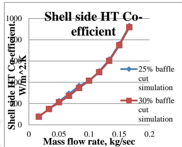
Fig. 22: Shell side heat transfer co-efficient variation for baffle cuts
