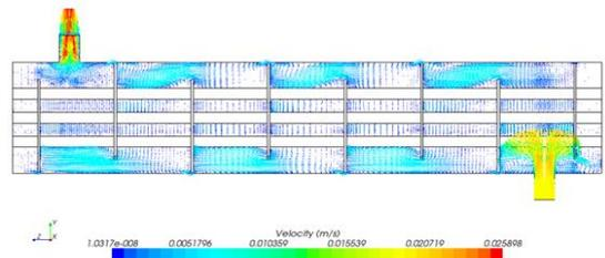
Fig. 7: Velocity vectors across section plane for 60 kg/hr
