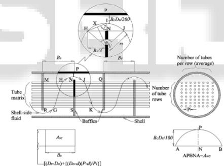
Fig. 4: Showing the actual flow pattern in shell-side
