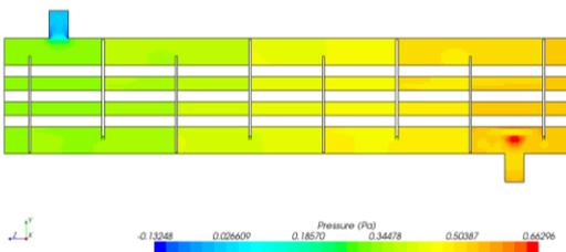
Fig. 6: Scalar contour of pressure across section plane for 60 kg/hr
