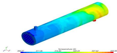
Fig. 11: Scalar contour of temperature for 60 kg/hr
