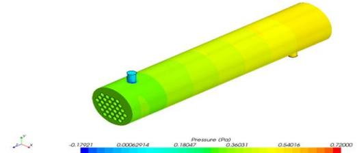
Fig. 8: Scalar contour of pressure for 60 kg/hr
