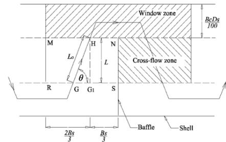
Fig. 3: Delination of cross-flow and window zones
