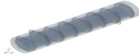
Fig. 1: The model with 8 baffles
