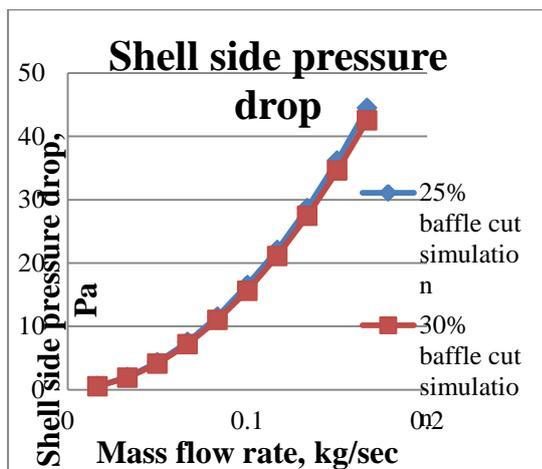
Fig. 20: Shell side pressure drop variation for baffle cuts
