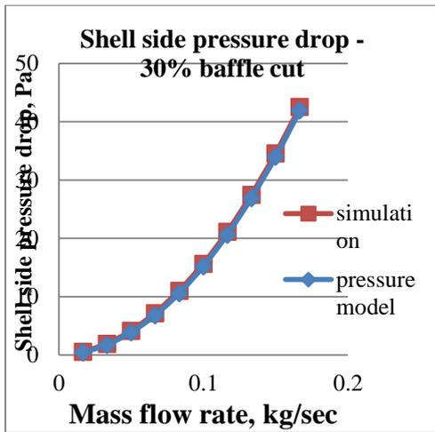
Fig. 18: Shell side pressure drop as a function of mass flow rate for 30% baffle cut
