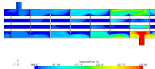
Fig. 10: Scalar contour of temperature across section plane for 60 kg/hr
