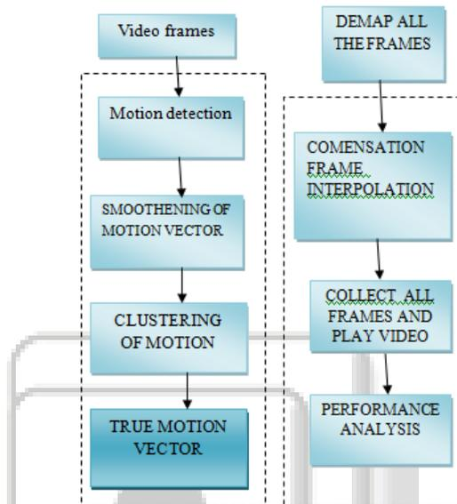
Fig.2 block diagram of true motion estimation and compensated temporal frame interpolation
