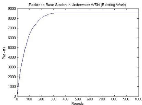
Fig. 7: Packet Transmitted to base Station(Existing Approach)
