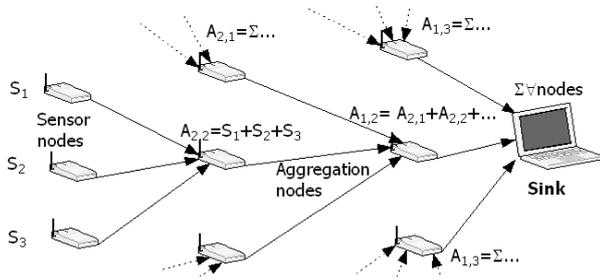
Fig. 1: in-network data aggregation
