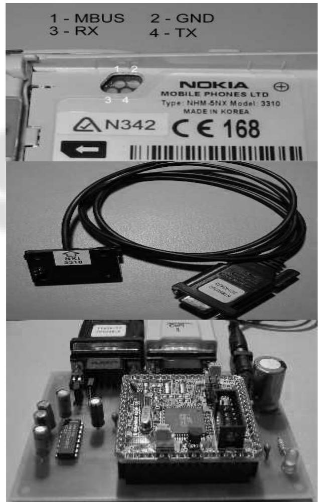
Fig.5: INTERFACING MICRO-CONTROLLER WITH MOBILE PHONE
