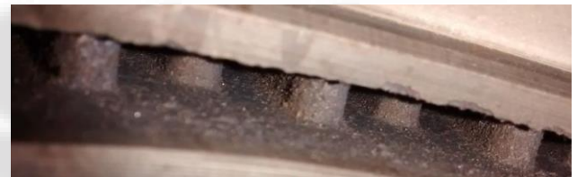
Fig. 5: Rotor42 have long length and short length vanes.
