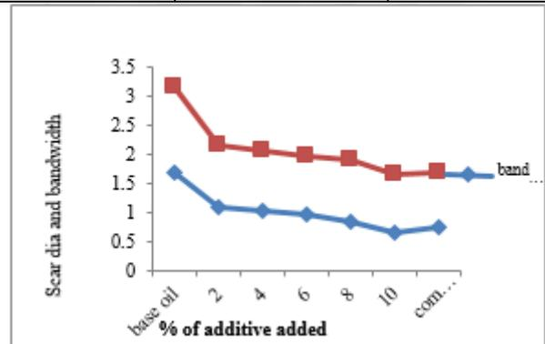
Fig. 3.2a: variation of scar dia and bandwidth with the addition of additive
