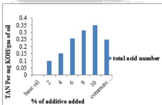
Fig 3.3: variation of TAN with addition of additive
