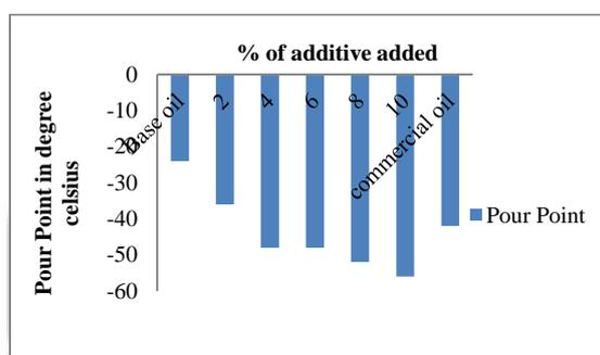
Fig 3.4: variation of pour point with addition of additive
