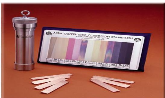
Fig. 3.6: Copper Strip Corrosion Strips And Test Bomb
