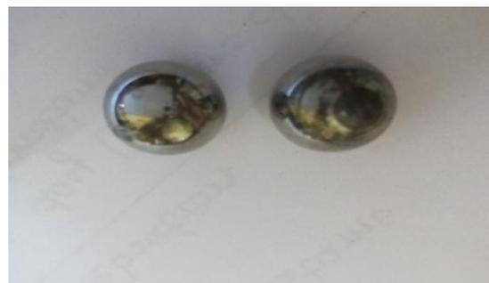
Fig. 3.2b: Balls with Scar and Band Width for the fourth ball
