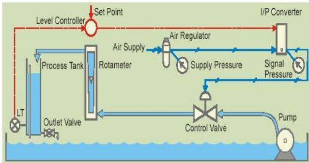
Fig. 2.2. Process diagram of Liquid Level System
