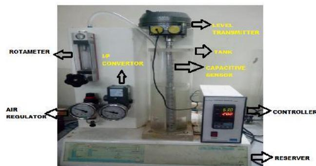
Fig. 2.1 Liquid Level System
