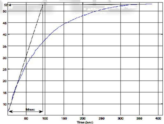
Fig. 3.1 FOPDT model identification for liquid level system
