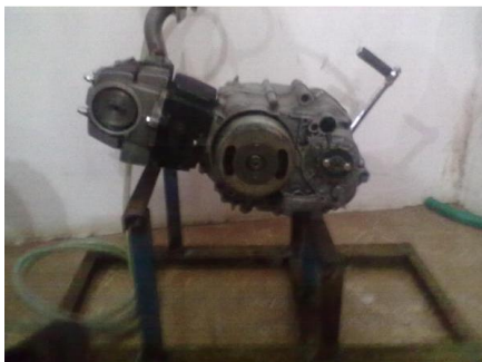
Fig. 3: Four stroke engines convert into two stroke engine
