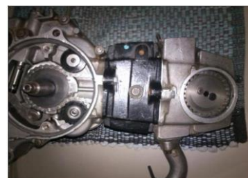
Fig. 12: Modified Crank Shaft Timing Gear
