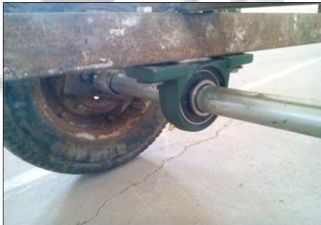
Fig. 14: shows mounting of rear shaft to chassis
