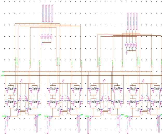
Fig. 9: Nibble Multiplexer using proposed logic.
