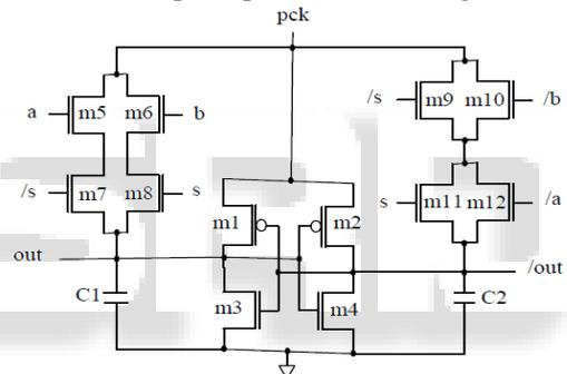
Fig. 5: 2:1 Multiplexer in PFAL logic
