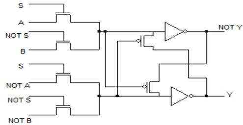
Fig. 4: 2:1 Multiplexer in EEPL logic
