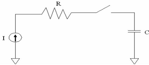
Fig. 2: Discharging Process of Adiabatic Logic
