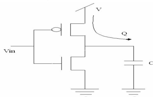
Fig. 1: Adiabatic Logic Circuit
