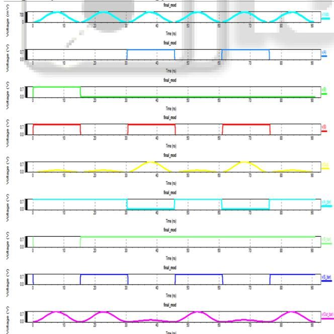
Fig. 7: Output Waveforms of 2:1 Multiplexer
