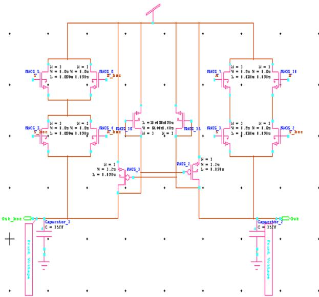
Fig. 6: Schematic of Proposed 2:1 Multiplexer
