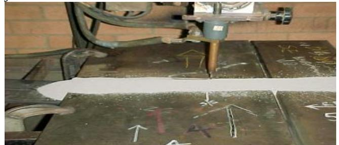
Fig.1: Principle of sub murg arc welding
