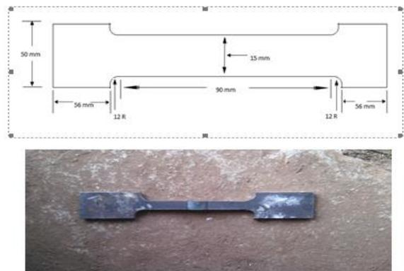
Fig. 3: sample specimen for tensile test
