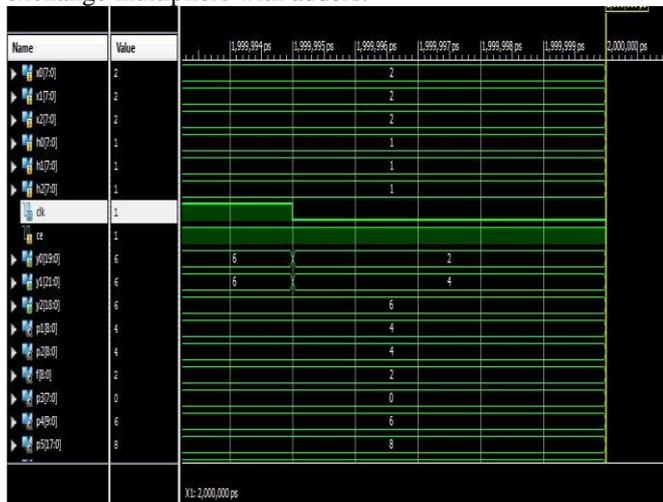
Fig.3: ISIM-simulation of Heterogeneous Adder
