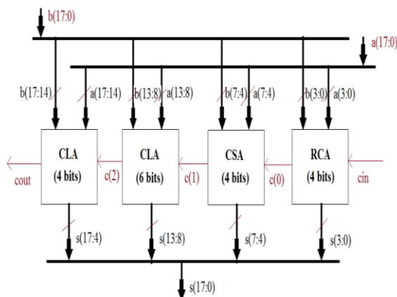
Fig. 1: 18-bit Heterogeneous adder
