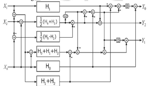
Fig. 2: Three-parallel FIR structure 3A.
