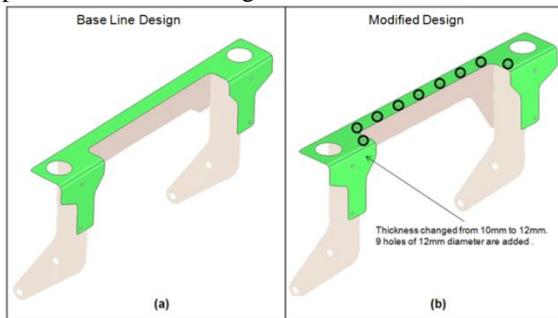
Fig. 9: Design Modification - 3 (a) baseline design (b) Modified design
