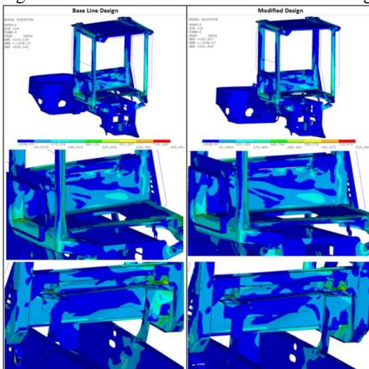
Fig. 5: von-Mises Stress Plot for Vertical Loading
