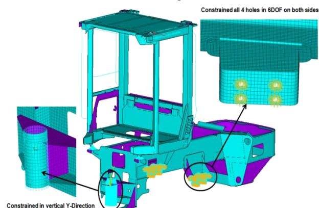
Fig. 3: Remote displace boundary conditions
