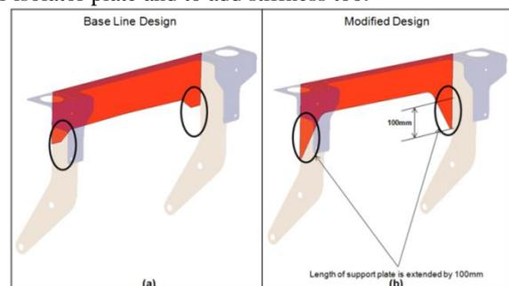
Fig. 8: Design Modification - 2 (a) baseline design (b) Modified design
