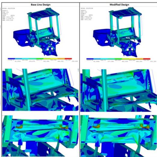
Fig. 4: von-Mises Stress Plot for Lateral Loading
