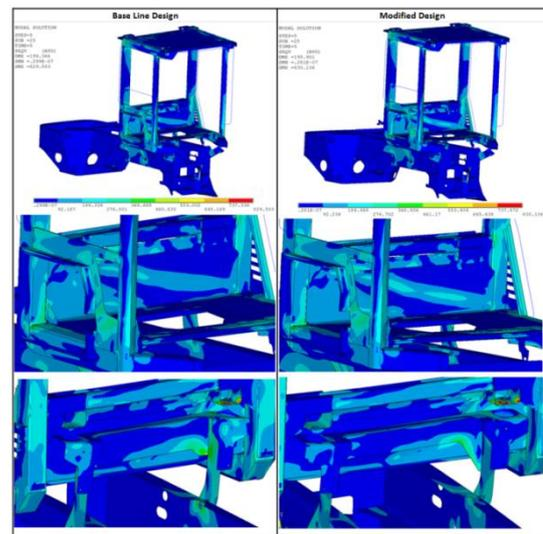
Fig. 6: von-Mises Stress Plot for Longitudinal Loading
