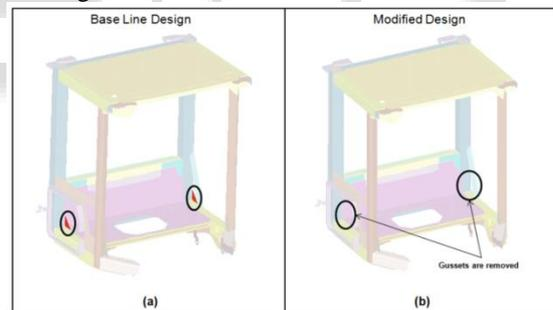
Fig. 7: Design Modification - 1(a) baseline design (b) Modified design
