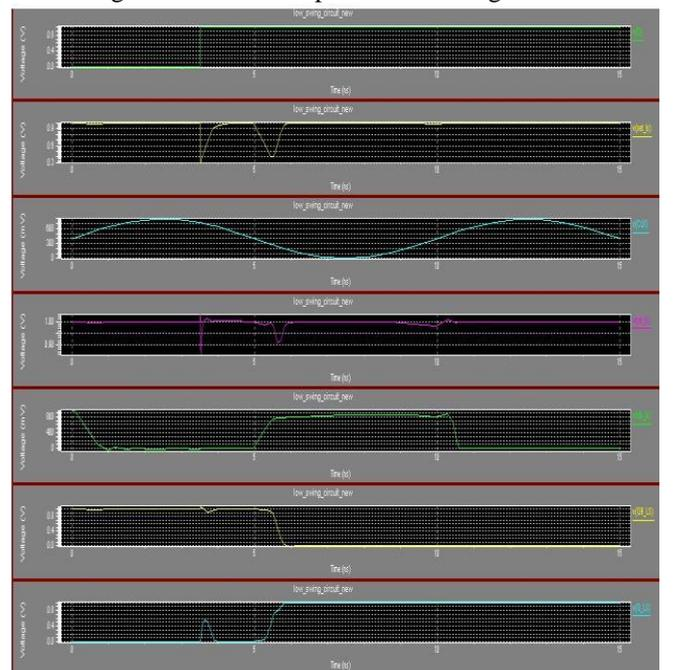
Fig. 5: Simulated output for low swing circuit
