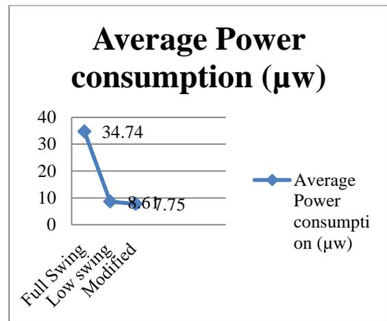
Fig. 8: Power dissipation graph for various circuits
