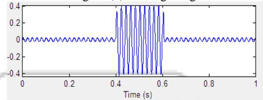
Fig. 17(b): Voltage Injected By DVR With hysteresis controller
