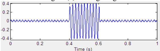
Fig. 18(b): Voltage Injected by DVR With hysteresis controller
