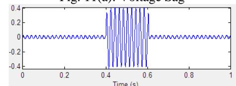
Fig. 11(b): Voltage Injected By DVR With hysteresis controller
