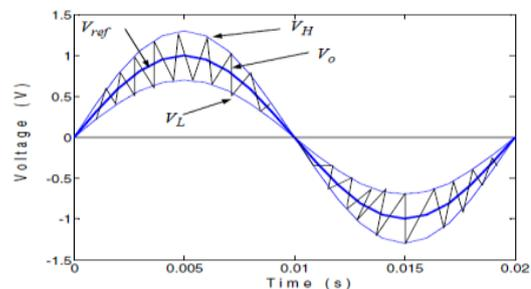
Fig. 6: Principle of operation of hysteresis voltage controller [8]
