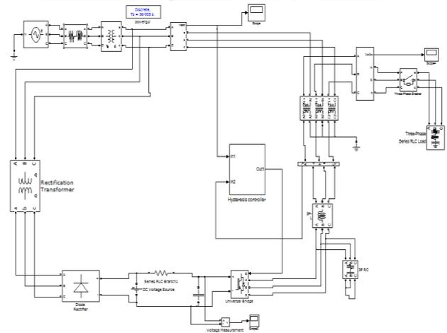
Fig. 16: Matlab/ Simulink of proposed scheme with Hysteresis controller
