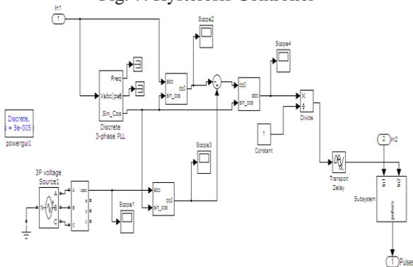
Fig. 8: Hysteresis Voltage Control Technique
