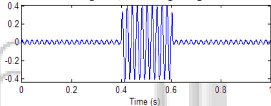
Fig. 12(b): Voltage Injected By DVR With hysteresis controller
