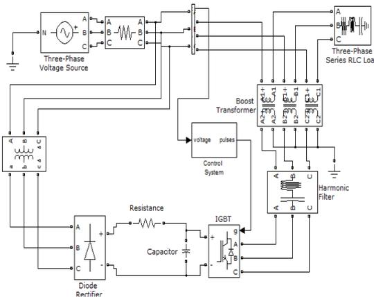
Fig. 4: DVR with no energy storage system and supply side connected rectifier
