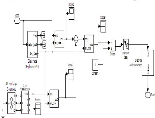
Fig. 5: Simulink model of feed forward control technique
