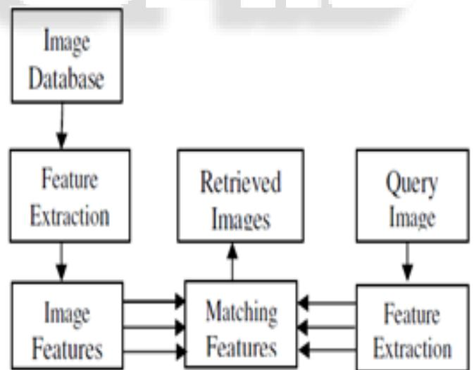
Fig 1: The generalized block diagram of system [1]
