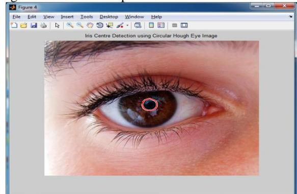
Fig. 5: Pupil Detection using Circular Hough Transform
