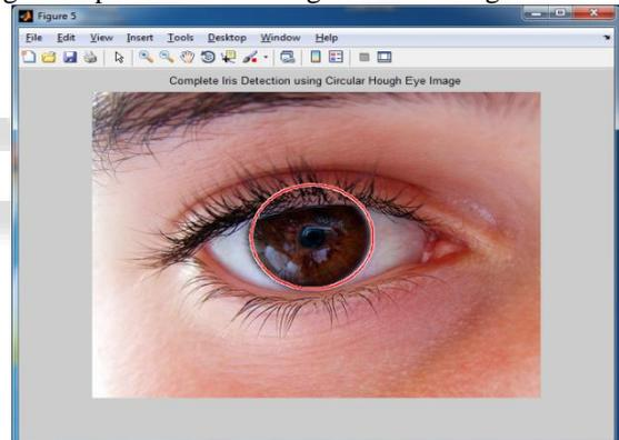
Fig -6: Iris Detection using Circular Hough Transform
