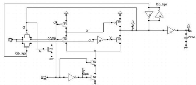
Fig. 1: CLOCKED PAIRED SHARED FLIP-FLOP (CPSFF)
