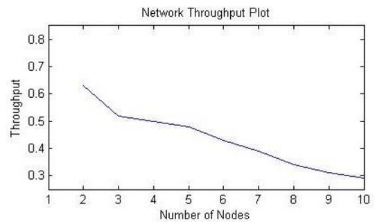
Fig. 1: Network throughput plot for Enhanced hybrid scheduling algorithm.
