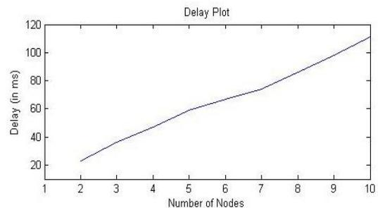
Fig. 2: Network delay plot for Enhanced hybrid scheduling algorithm.
