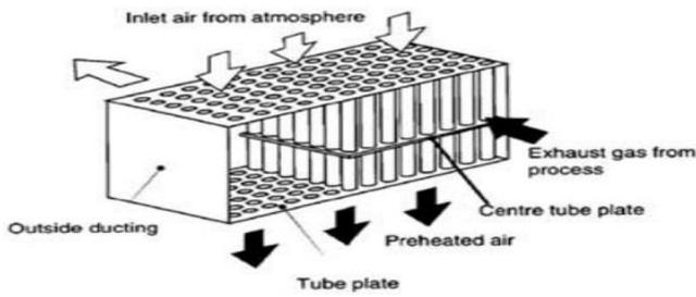
Fig. 1: Waste Heat Recovery using Recuperator
