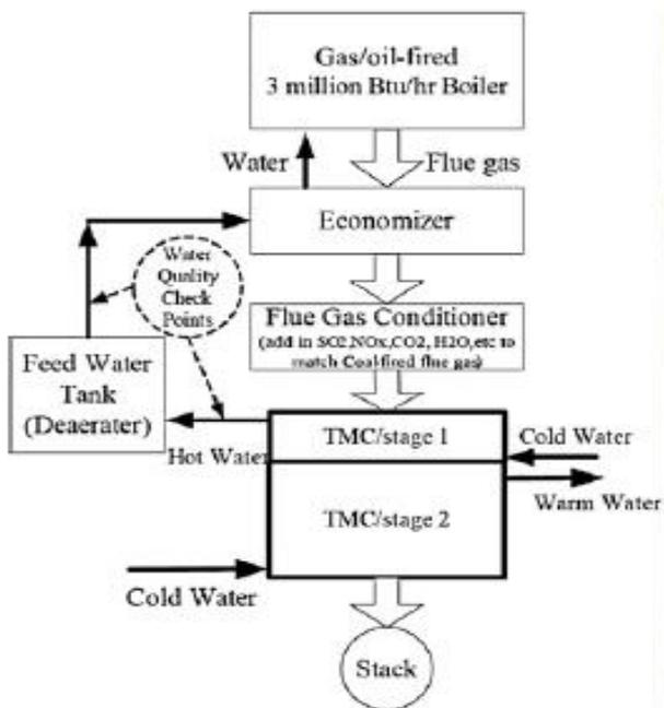
Fig. 10: Pilot-Scale TMC Test Setup Schematic
