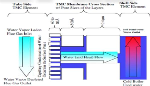
Fig. 6: TMC concept schematic
