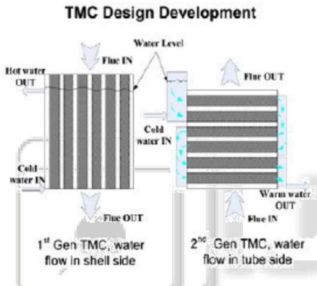
Fig. 7: New membrane module, 1st and 2nd gen TMC
