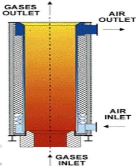
Fig. 2: Metallic Radiation Recuperator
