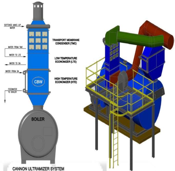
Fig. 8: Stacked installation design (left), and skid installation design (right)
