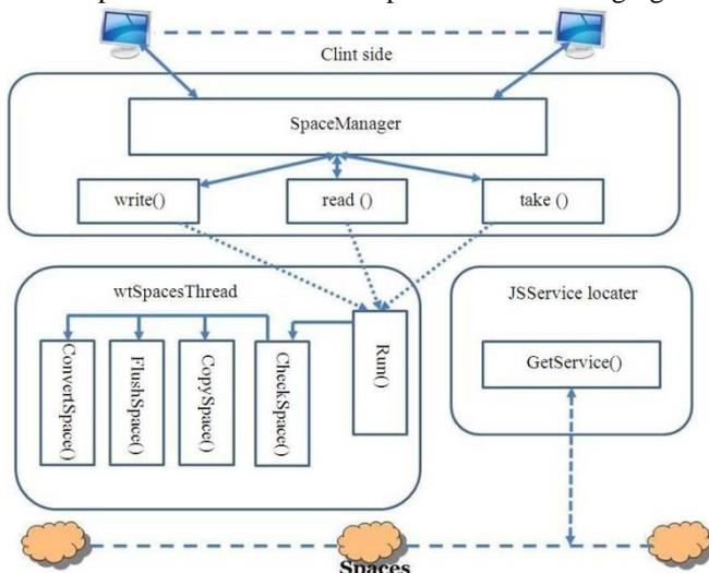
Fig. 6. FTJS internal structure
