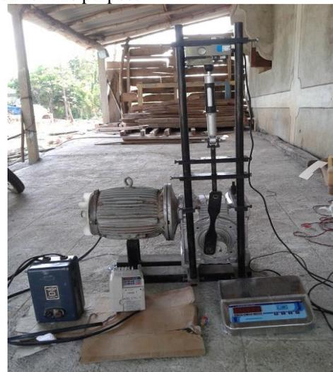
Fig 2: Shock absorber test rig.
