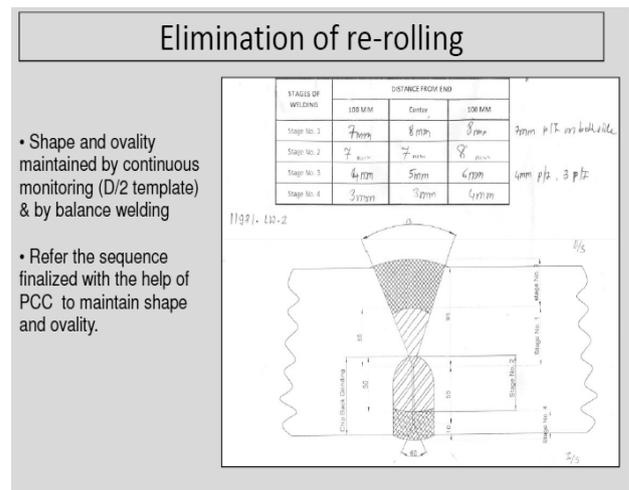
Fig.3: Data Monitoring during Welding
