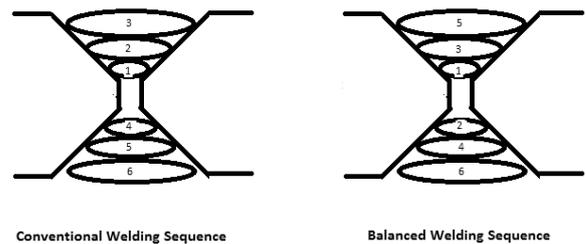
Fig.1: Difference between Conventional and Balanced Welding
