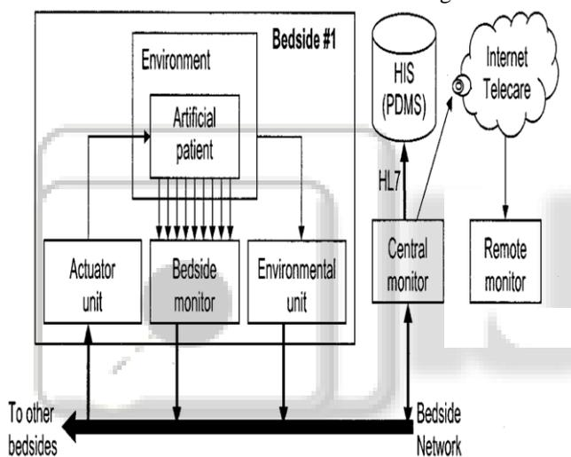
Fig. 1: Structure of the open architecture patient monitoring system
