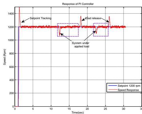
Fig. 8: Actual response of PI controller implemented on Arduino
