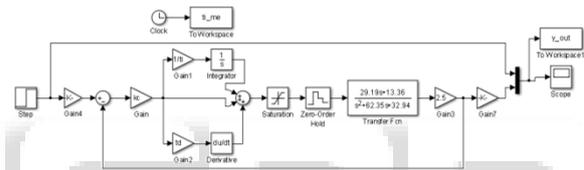
Fig. 3: PI controller for single Motor system
