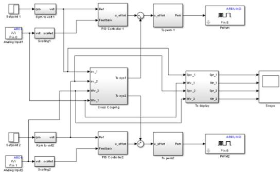
Fig. 10: Simulink model for cross couple system
