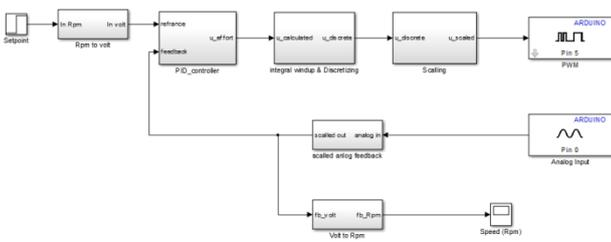
Fig. 9: Simulink model running on Arduino
