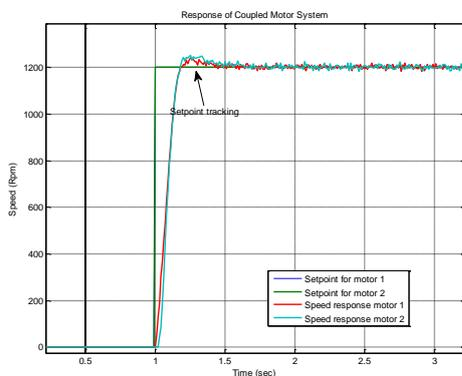
Fig. 12: near view of coupled system for set point of 1200 rpm
