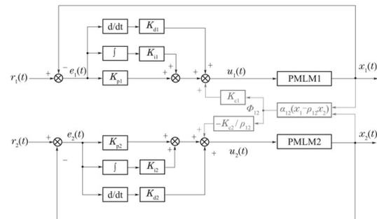
Fig. 2: Block Diagram of Cross coupling
