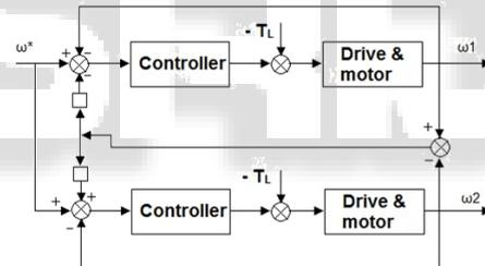
Fig. 1: Structure of cross couple technique
