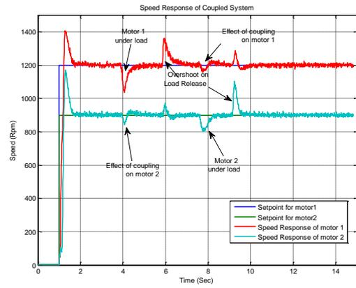
Fig. 13: Coupled system for different set point of 1200 & 900rpm
