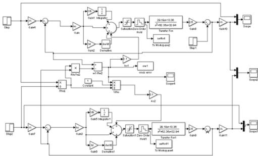
Fig. 5: Cross coupling of two DC motor
