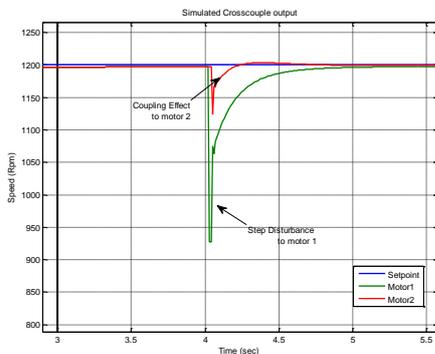
Fig. 7: Disturbance rejection or system under load change
