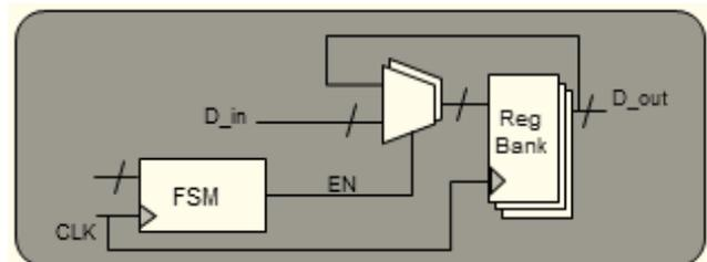
Fig. 1: Synchronous load enable Registers
