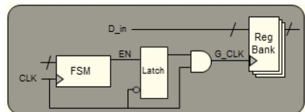
Fig. 2: Latch based Clock Gating
