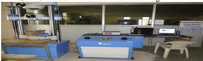
Fig. 2: Universal Testing Machine 600 kN capacity
