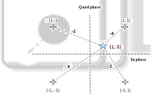
Fig. 9: Branch Metric Calculation using Euclidean Distance Approach
