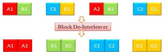
Fig. 7: Block De-Interleaver
