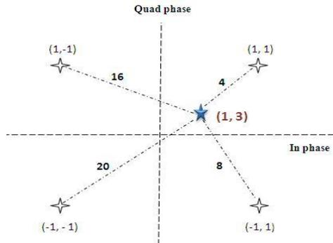
Figure 15. Distance Calculation Between Neighbour Points Using Conventional Method
