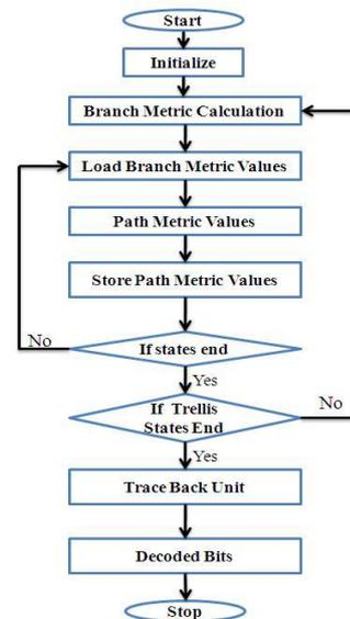
Fig. 16: Implementation Flow Of Viterbi Decoder
