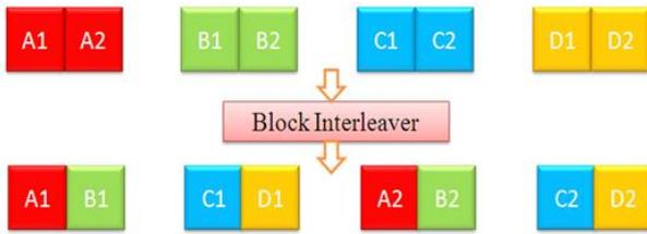
Fig. 3: Block Interleaver
