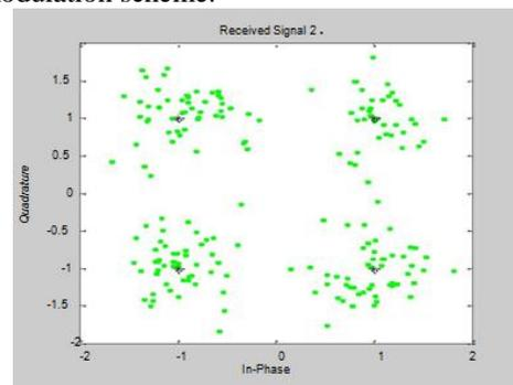
Fig. 13: Matlab Simulation Result For QPSK
