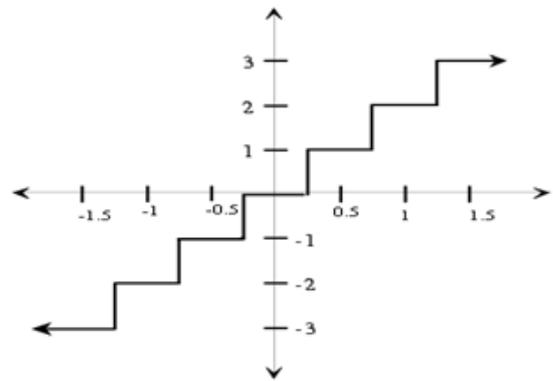
Fig. 6: Quantization Process
