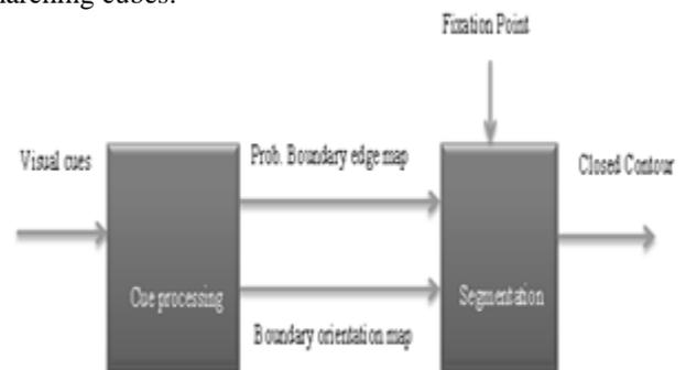
Fig. 1: shows the model of segmentation process
