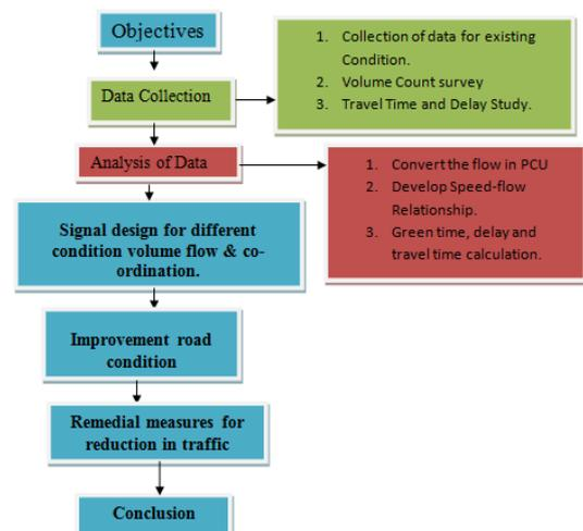
Fig. 1: Flow diagram of whole methodology
