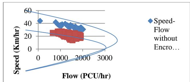
Fig. 1: Speed-flow diagram at bus stand to malpur cross road.[Ref.4]
