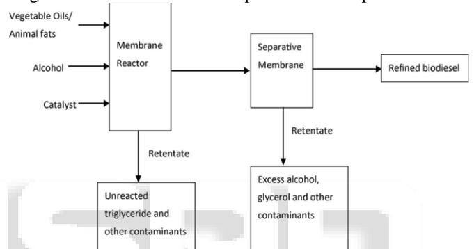
Fig. 3: Biodiesel production and purification using membrane technology.
