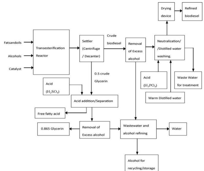
Fig. 2: Conventional biodiesel production and purification.
