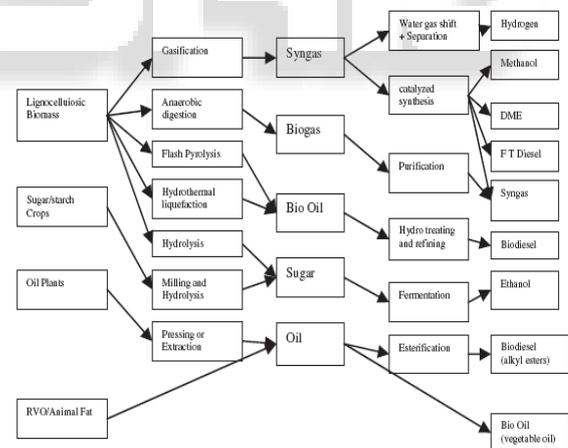
Fig. 1: Overview of conversion processes of Biofuels. Before any alternative fuel is to be used in existing systems the following factors need to be taken care of:
