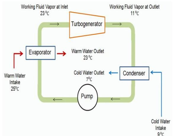
Fig. 2: Schematics diagram of traditional closed OTEC operation [3]
