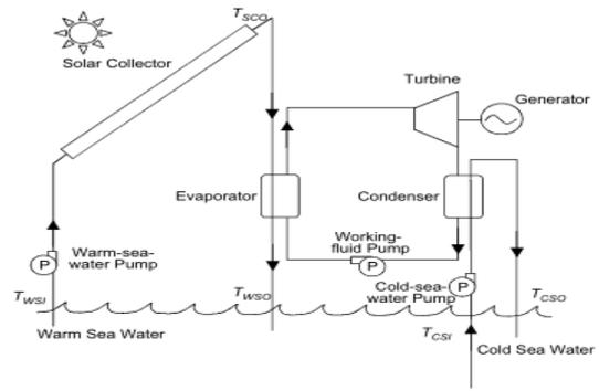
Fig. 4: Schematics of Indirect SOTEC operation [1]
