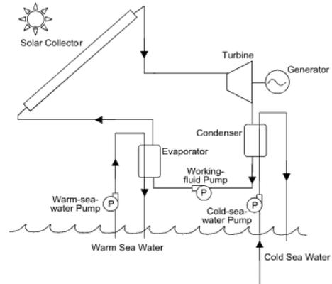
Fig. 5: Schematics of Direct SOTEC operation [1].
