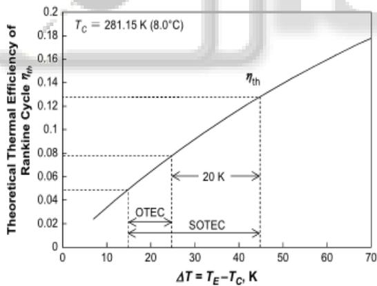
Fig. 3: Curve of efficiency of OTEC and SOTEC with the variation of temperature difference [1]
