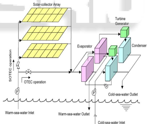
Fig. 6: Schematics of SOTEC Plant operation.
