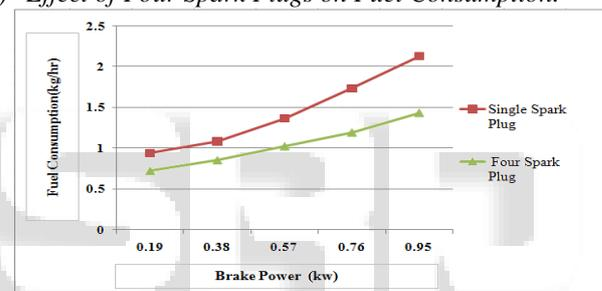
Fig. 1.1: Variations in Fuel Consumption with B.P.
