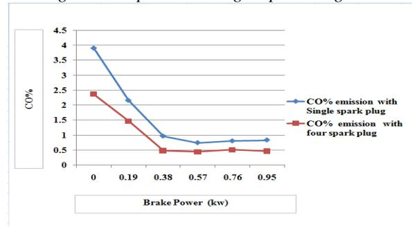
Fig. 1.6: Variations in Carbon monoxide (CO) emission versus Brake Power
