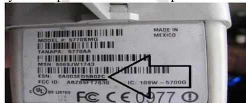
Fig. 2: ESN (Electronic Serial Number)
