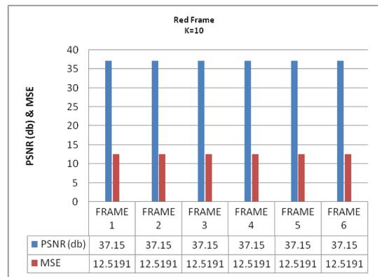
Graph 1.1(b): PSNR & MSE calculation in Performance analysis of watermarking techniques for Correlation based DCT.
